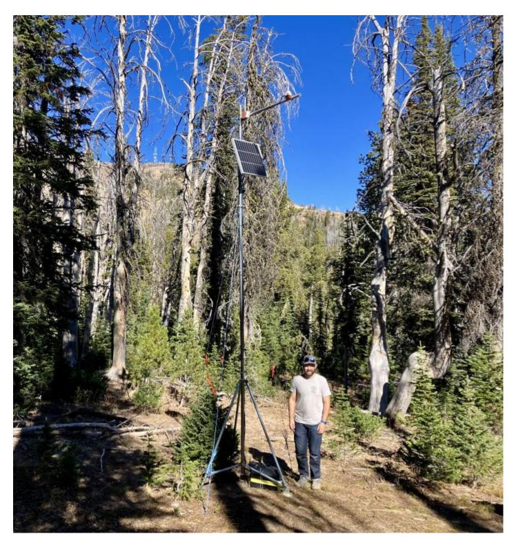
We completed the setup of a SNOdar snow depth sensor on Sawtelle Peak in the Centennials on Wednesday 10/19. Forecaster Ian Hoyer for scale.
